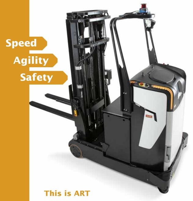
Rocla's automated reach truck is designed to operate in an aisle width of 3 meters. New and innovative software and sensor technology increase the load handling speed considerably. The agile turning radius and lifting capability of 10 meters fulfill the requirements of the most common warehouse environments.
